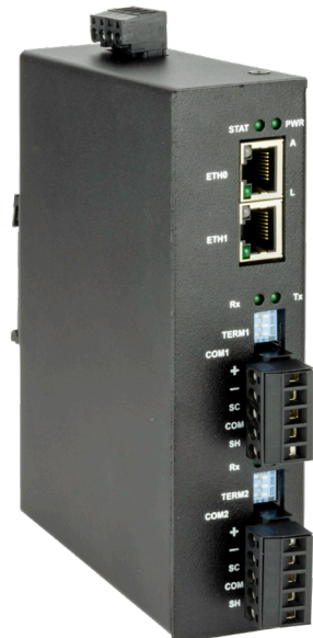
PI Platform – Dual Ethernet and EIA-485 connectivity
