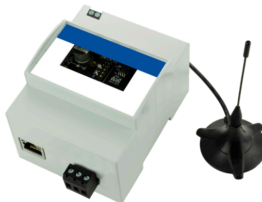
SBCti and hat in 4M enclosure for a wireless gateway
